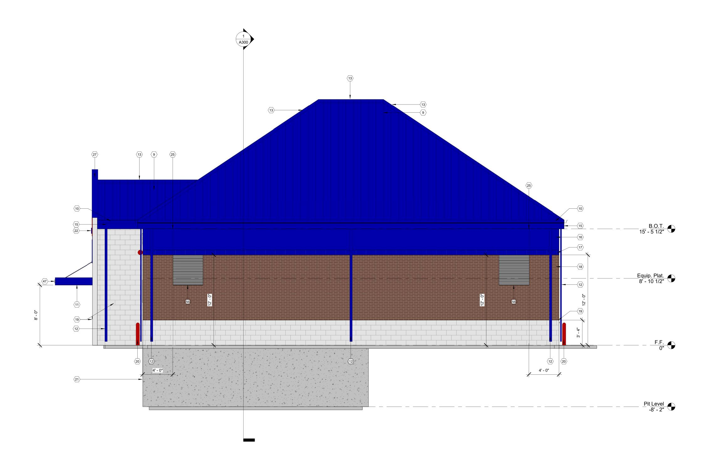
Note: Align top of exterior wall packs with bottom of banding at 12'-0" a.f.f. Top of emergency lighting at exit doors to be aligned with top of door frame. Do not locate exterior wall packs on side of building that contains illuminated lightbars or sconces by others.
