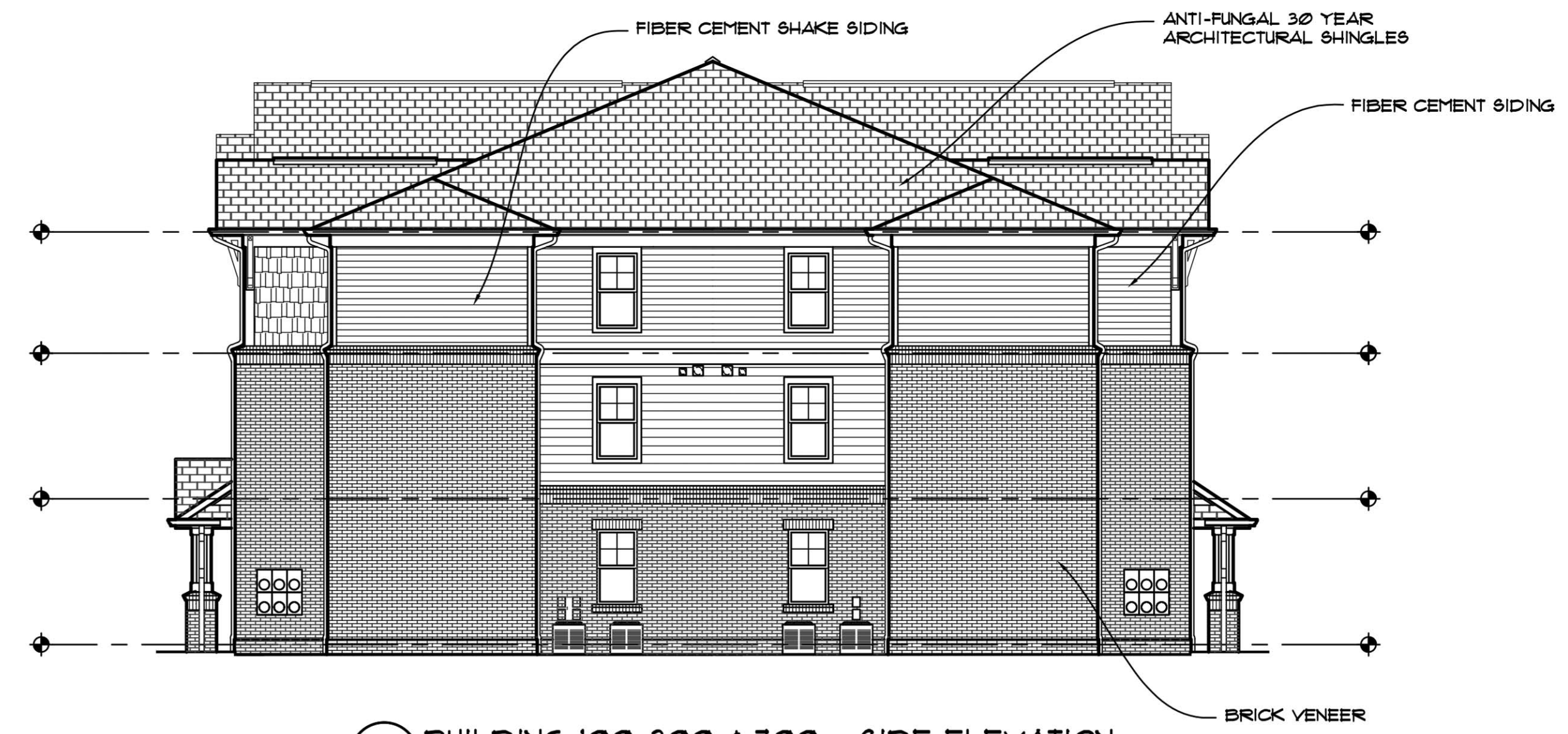
3 BUILDING 100, 200 & 700 - SIDE ELEVATION 1/8" = 1'-0"
