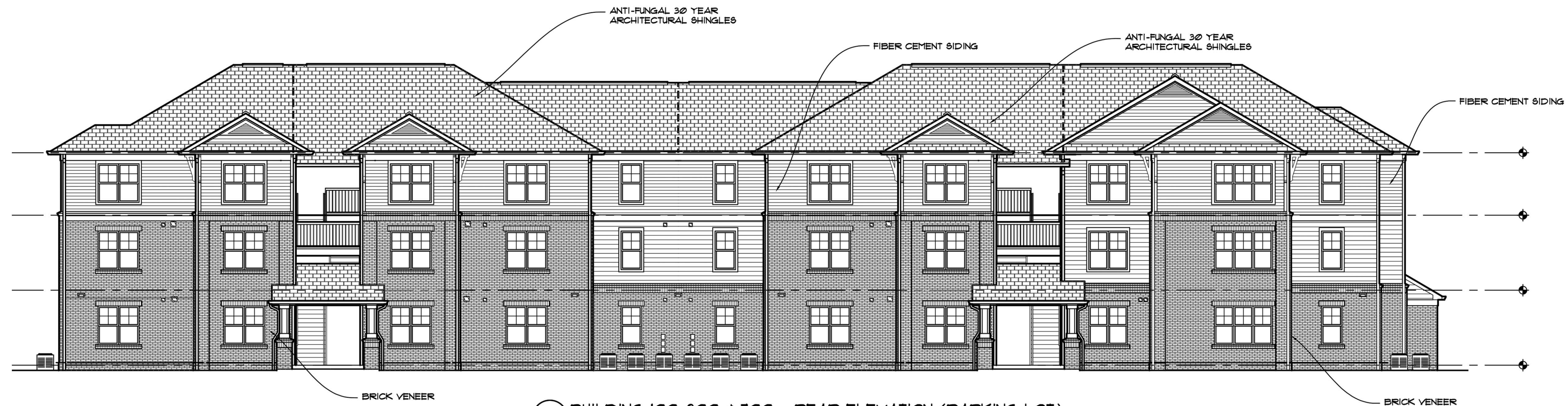
2 BUILDING 100, 200 & 700 - REAR ELEVATION (PARKING LOT) 1/8" = 1'-0"
