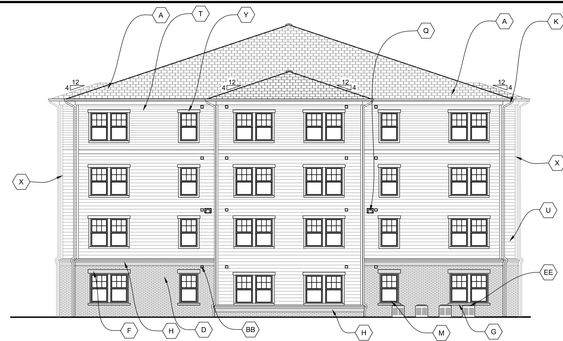
3 BUILDING 100 - RIGHT SIDE ELEVATION 3/32" = 1'-0"
