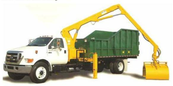
The Brush Hawg is a truck mounted knuckle boom loader that provides streetside collection of brush and limbs.
