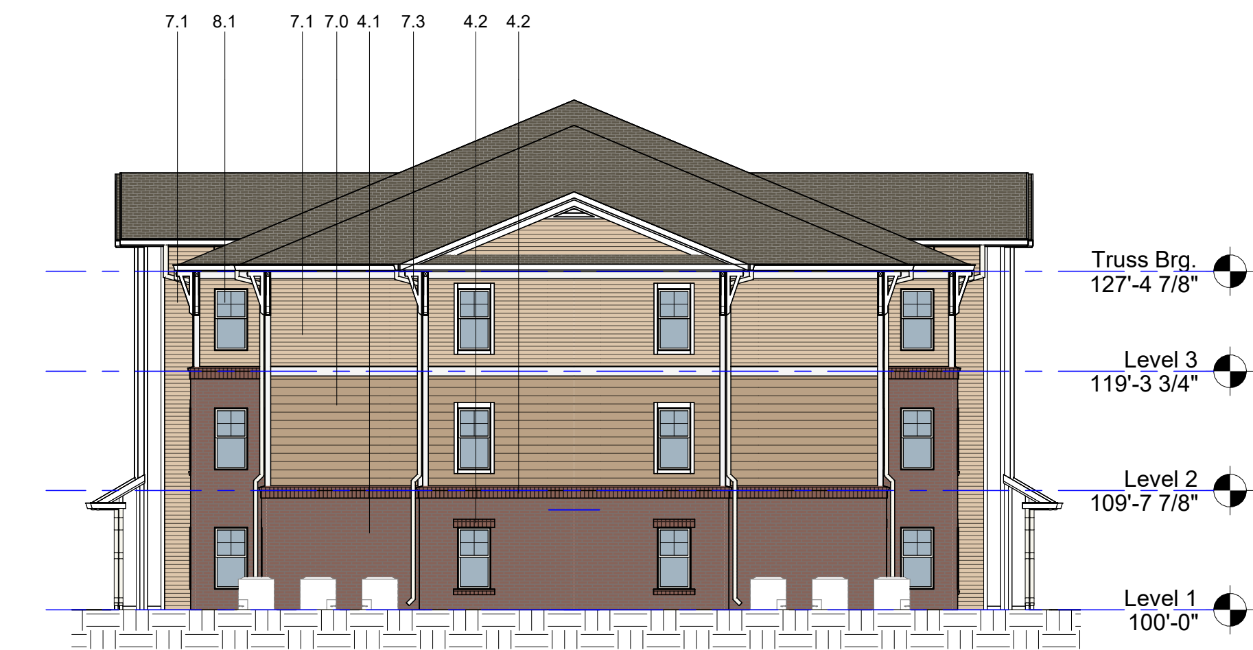
③ Building Type X - Left Elevation 3/32" = 1'-0"
