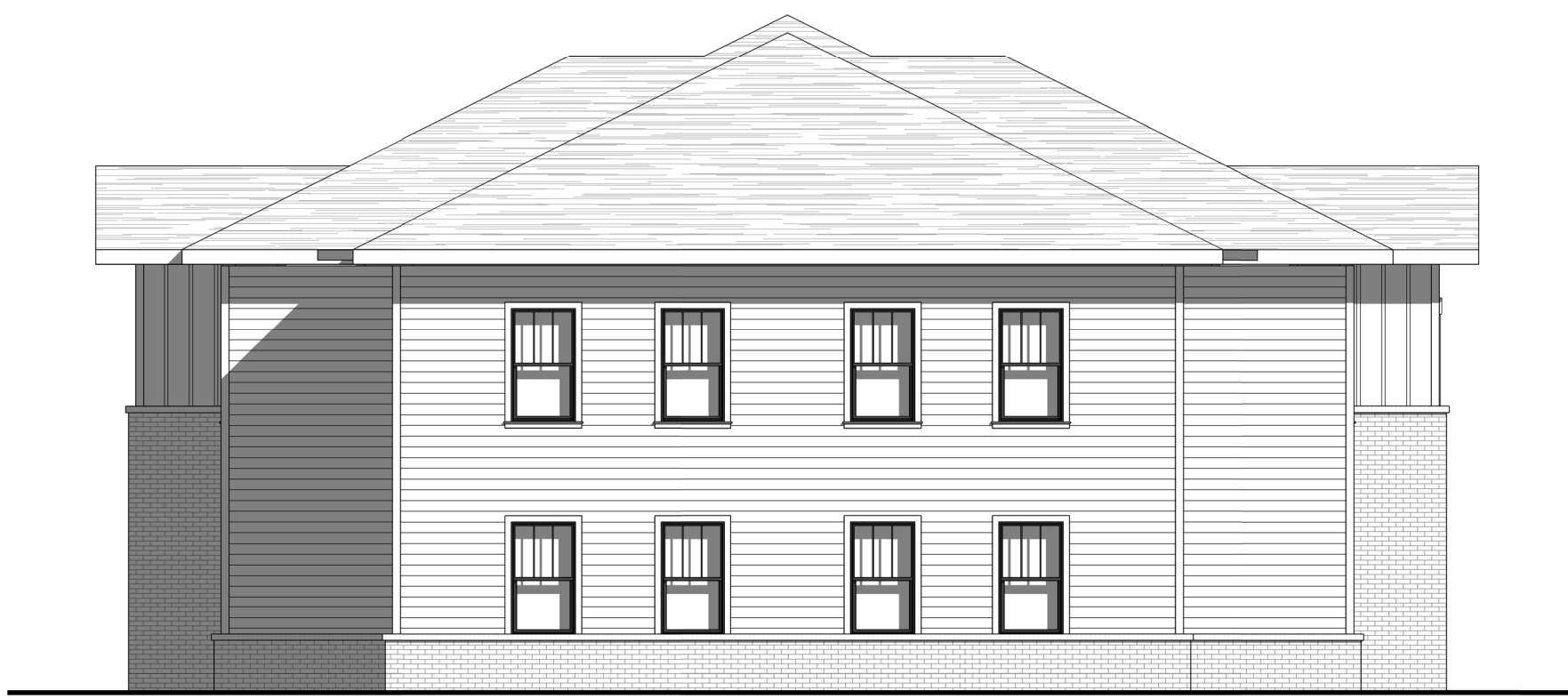
3 ELEVATION - BLDG G (EAST) SCALE: 1/8" = 1'-0"
