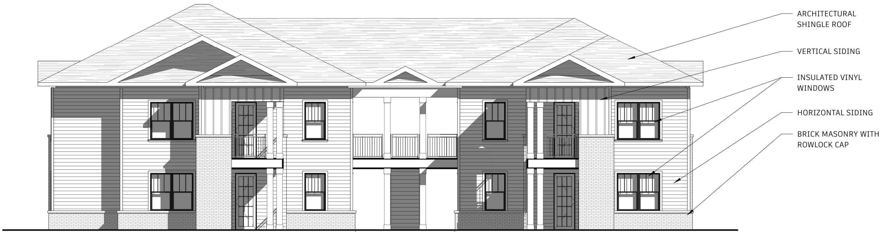
4 ELEVATION - BLDG A (NORTH) SCALE: 1/8" = 1'-0"
