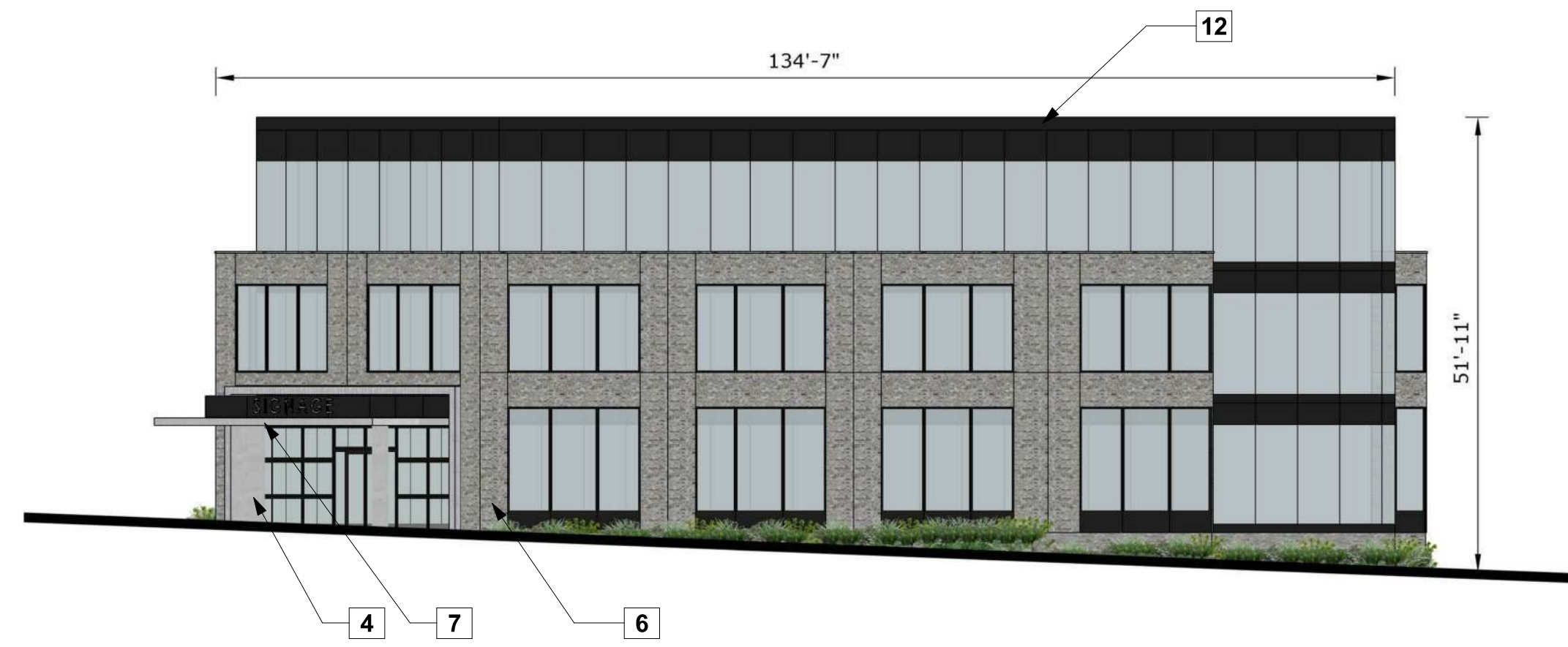
4 OFFICE - WEST ELEVATION 1/16" = 1'-0"
