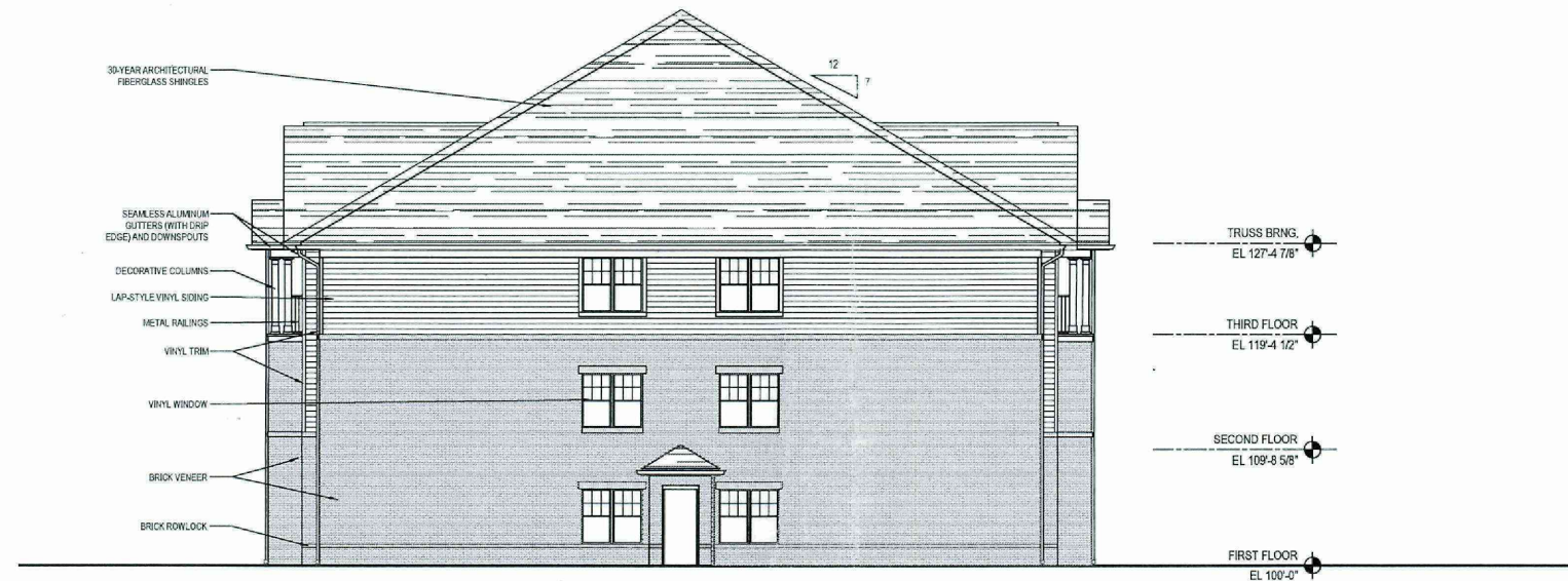
side elevation (bldg 'A' & 'A1')
