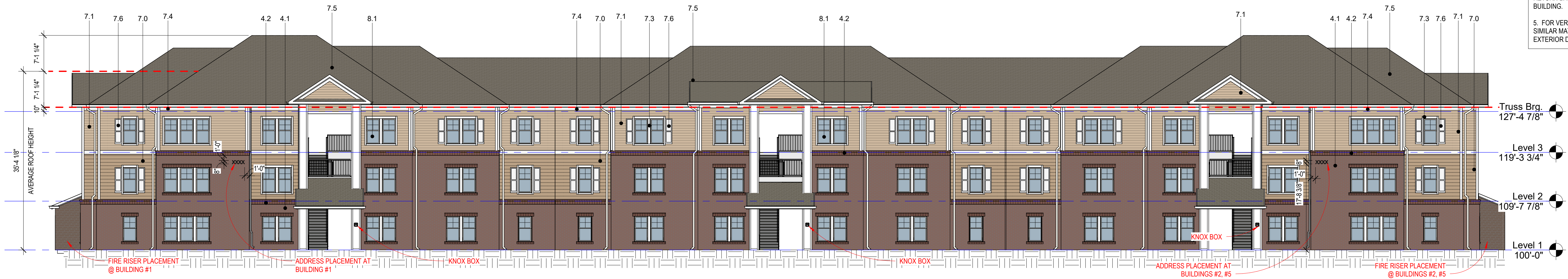
1 Building IX - Front Elevation 3/32" = 1'-0"
