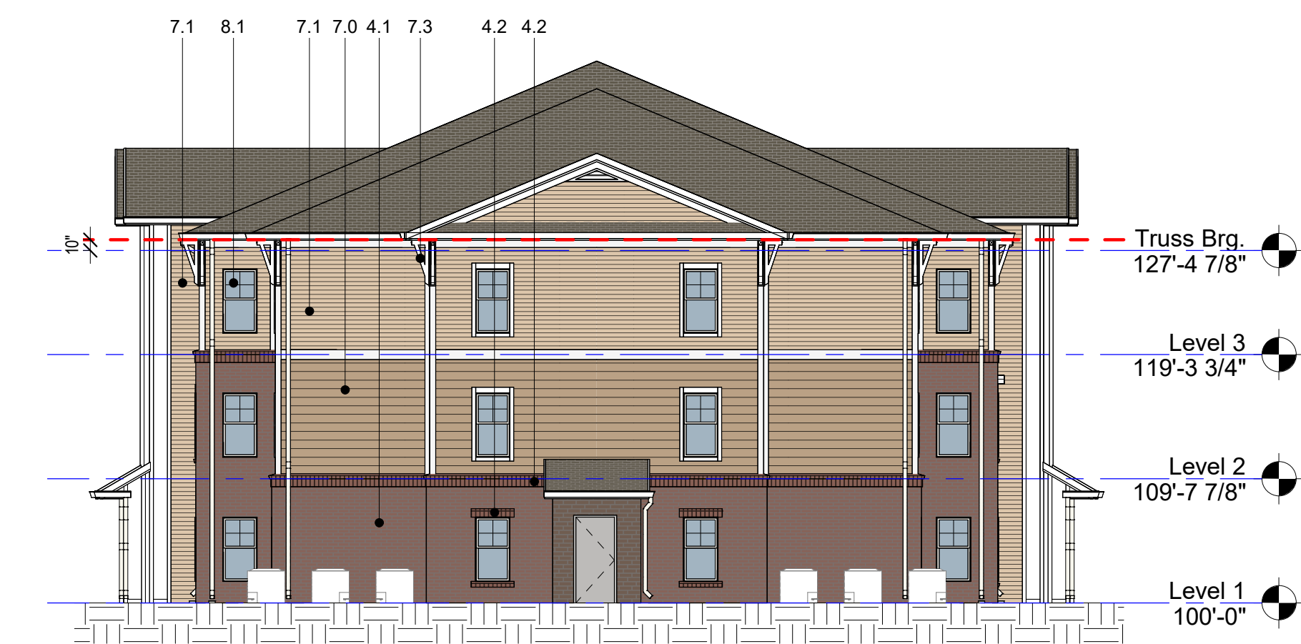
③ Building Type X - Left Elevation 3/32" = 1'-0"
