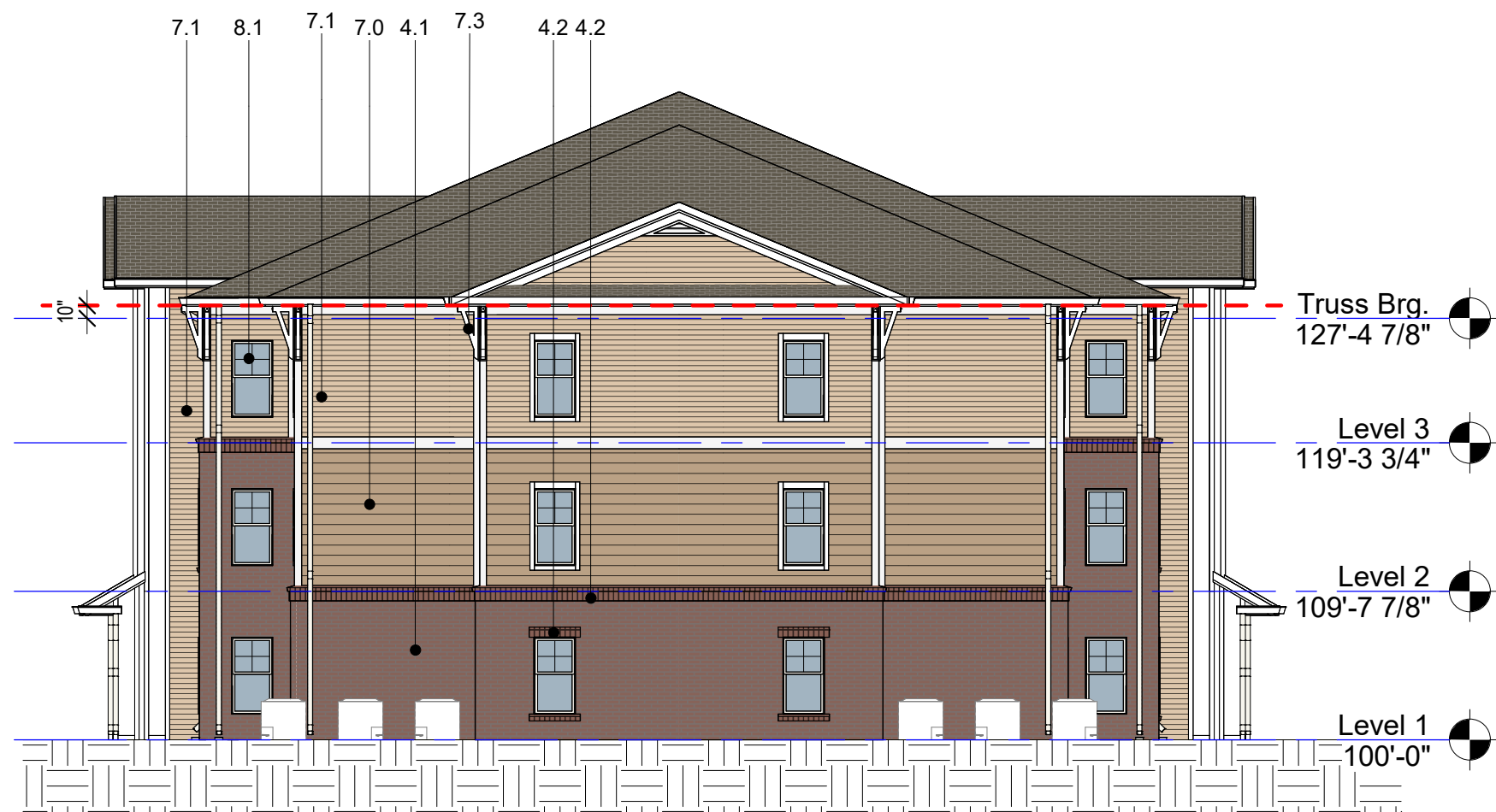
④ Building Type X - Right Elevation 3/32" = 1'-0"
